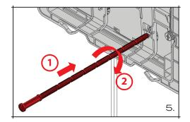
Test the depth needed for the flush rods by measuring how much of the rod needs to be broken off to protrude enough (step 7.) from the plate as well as having enough thread to attach to the flush mechanism without restricting on rear of the cistern.
